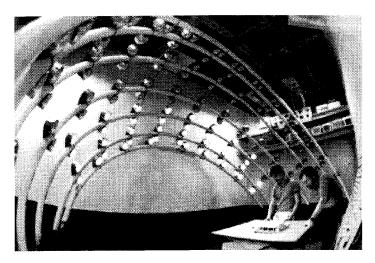
FIG. 2 This type of heliodon uses multiple lamps to simulate the daily and annual motion of the sun. For latitude adjustment the model table can be tilted a maximum of 10 degrees each way.
