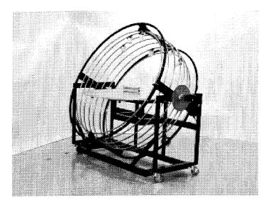
FIG. 3 The Sun Emulator simulates our real-world experience by keeping the building model stationary while the lights move to simulate all of the sun's apparent motion across the sky.
